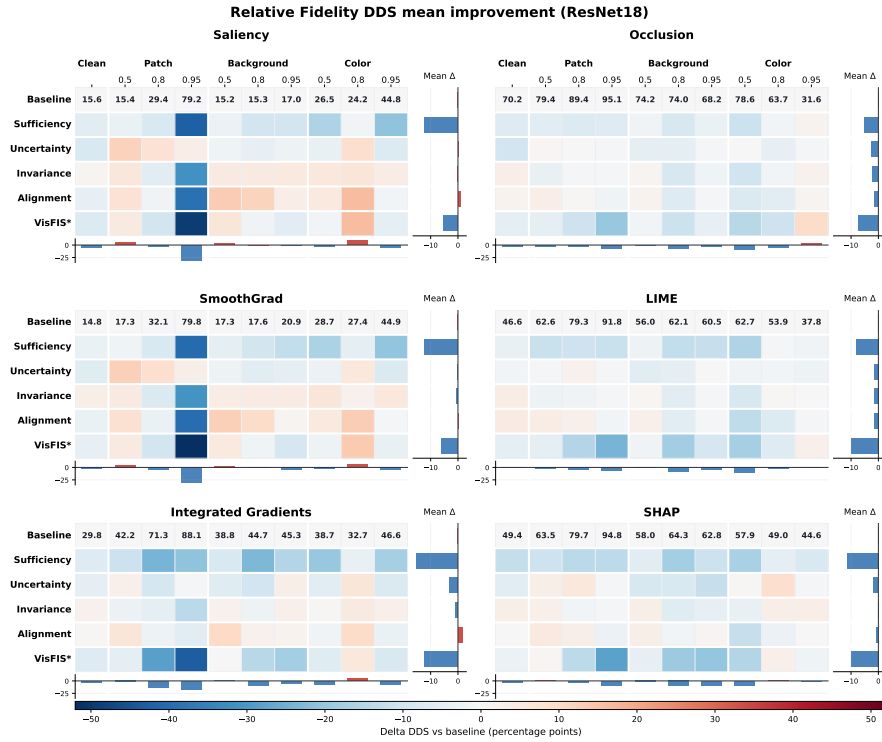
Fig. 4. RQ4. Relative ResNet18 fidelity change measured by DDS with mean replacement. \lambda^* is selected by highest \text{Test}_{\text{rand}} accuracy as in RQ1. Columns group shortcut types and correlations p , rows show objectives, and panels correspond to post-hoc explanation methods. Baseline DDS values are shown above each column.
